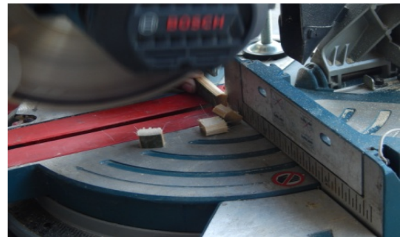
Fig. 2. preparation of Bamboo aggregates by Cross cutter
