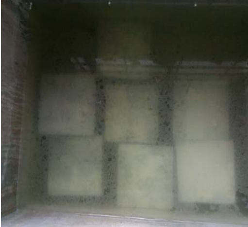
Fig. 4. Curing of cubes
