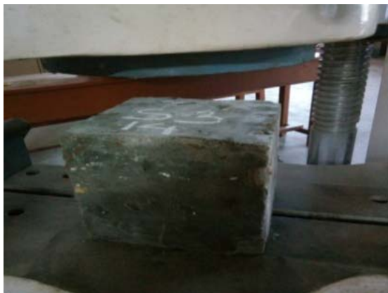
Fig. 6. Cubes placed under UTM
